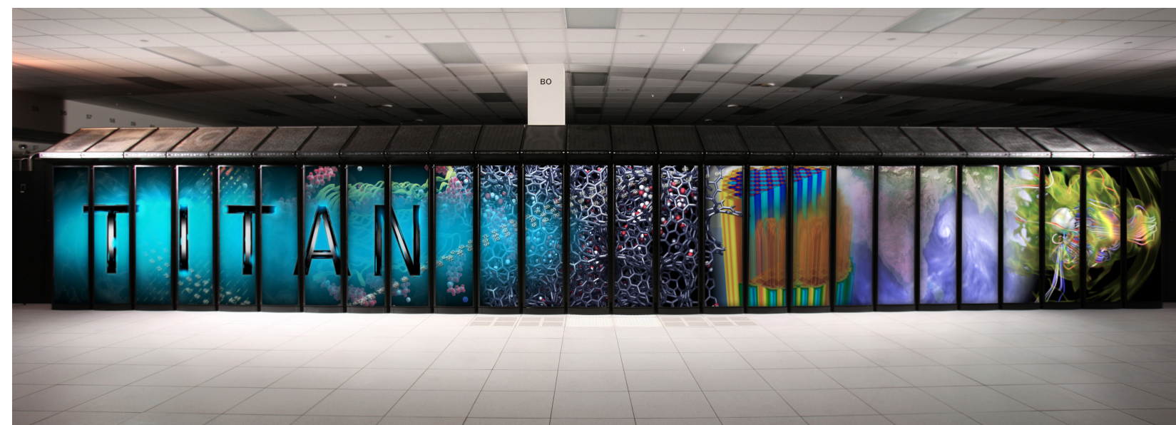
With a peak speed of over 20 petaflops (over 20,000 trillion calculations per second), Titan is a supercomputer composed of 299,008 AMD Opteron cores supported by additionally 18,688 Nvidia Tesla K20 GPU accelerators located at Oak Ridge National Laboratory, is one of the world's fastest supercomputers for unclassified research. Capable of simulating physical systems with heretofore unfeasible speed and accuracy.
